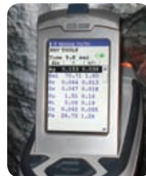
Instantaneous geochemical data in the field with Thermo Scientific NITON XL3 Analyzers.
